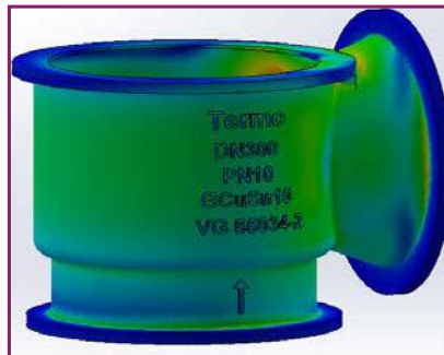
Angular Globe Valve Thermal and Mechanic Analysis
