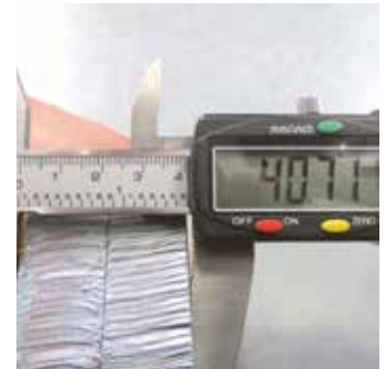
Carbon Steel Max. Cutting Thickness: 35 mm
