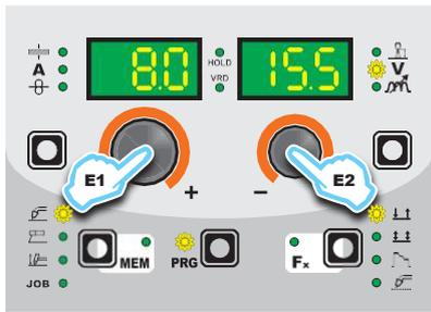
The HOLD function can be terminated ahead of time even while once again starting the welding. Once 15 seconds have passed (HOLD FUNCTION) the control panel goes back to the PRESETTING phase.
