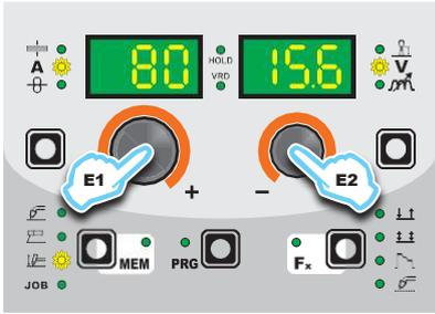
The HOLD function can be terminated ahead of time even once again starting the welding. Once 15 seconds have passed (HOLD FUNCTION) the control panel goes back to the PRESETTING phase.
