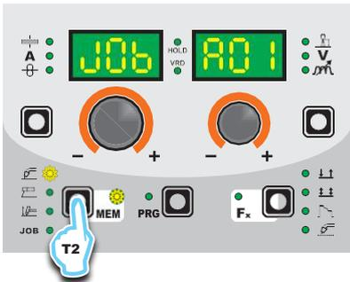
To be able to choose another automatic welding point (JOB) that is free for saving the data, simply turn one of the two ENCODER (E1-E2) knobs until you reach the required point.
