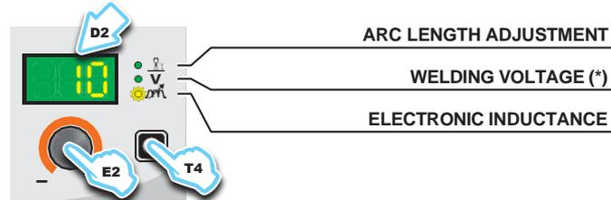
(\*) The parameter is pre-set by means of synergy and can be changed by varying the ARC LENGTH ADJUSTMENT parameter.
