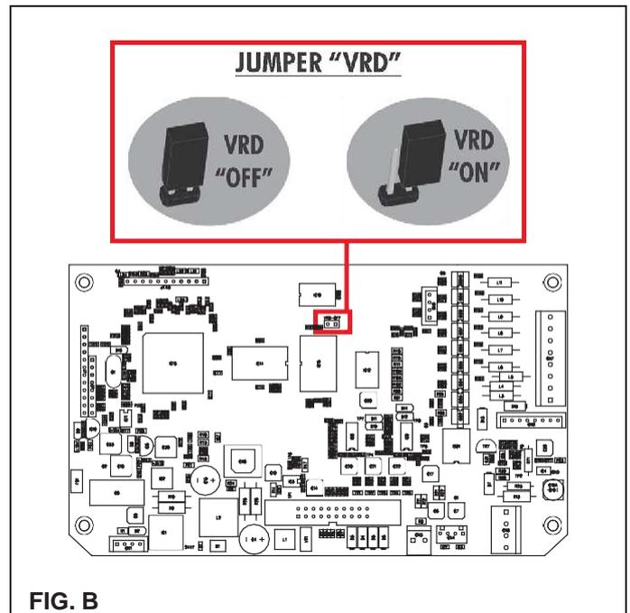
During the welding phase, this LED becomes RED, which however does not indicate a malfunctioning of the welder but the fact that the VRD device is in function and, at the conclusion of the welding operation, the tension will be reduced within a maximum greatest time of **0.3 seconds**.
