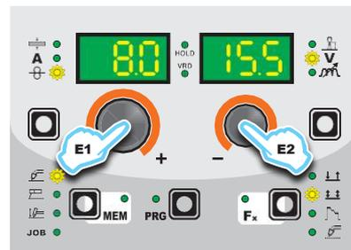
The HOLD function can be terminated ahead of time even while once again starting the welding.
