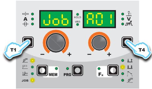
The control panel automatically goes to the first JOB saved or reads "no JOB" if no JOBS have been saved.
