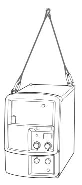
2. Lift the welding power source carefully paying attention to the balance by using lifting lug.
