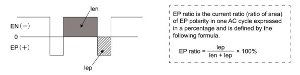
If you adjust the cleaning width, the EP ratio changes by 1% against the operation amount "1". The standard value of the EP ratio (the value at the center position "0") differs for each AC waveform, and the maximum value and the minimum value that can be set as EP ratio also differ.
