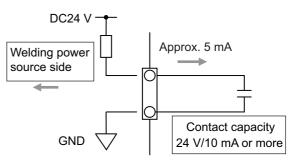
Output signal of the external connection terminal block Output signal is open collector output. Ensure to keep the maximum rated power of the transistor.
