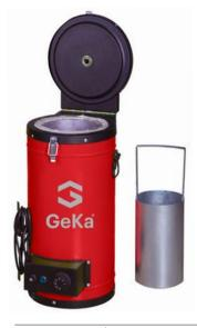
Its main function is to help keep electrodes manually at the desired temperature level between 60 and 200°C at the points of application. It can easily be used with all types of electrodes.
