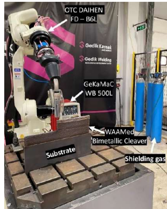
Figure 1. The robotic WAAM cell used to manufacture bimaterial cleaver
