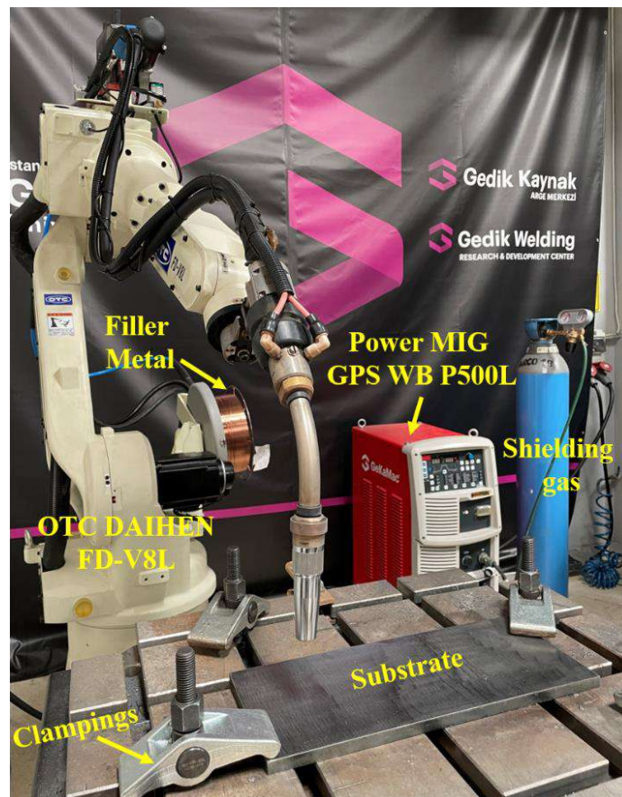
Figure 1. The robot cell for the robotic arc additive manufacturing process.
