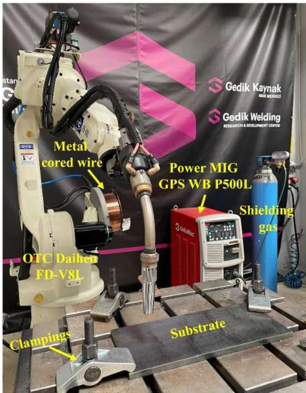
**Figure 2:** The experimental setup used for the wire arc additive manufacturing process.
