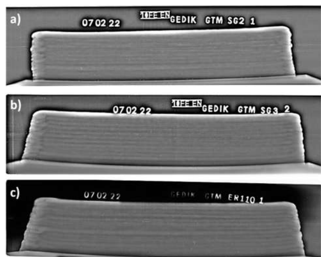
Fig. 4 Computed radiography test results of WAAM-produced parts using (a) SG2, (b) SG3, and (c) ER110 welding wires
