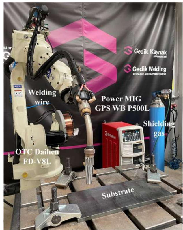
Fig. 1 The robotic cell for wire arc additive manufacturing (WAAM) process with GMAW welding machine
