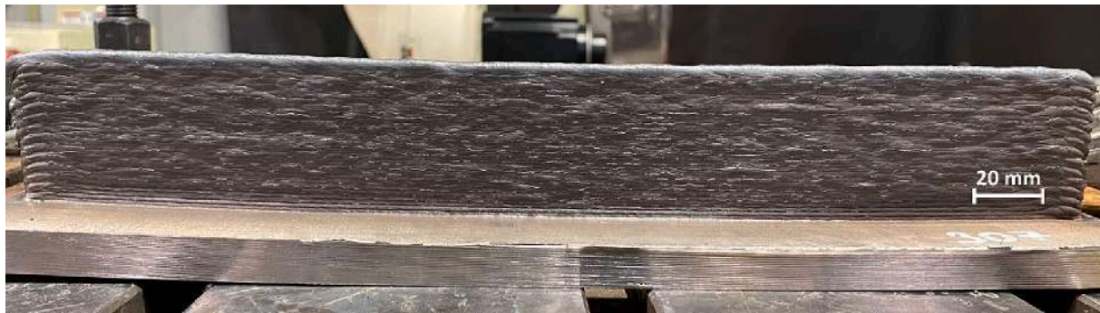
Fig. 1. Optical macrograph of ER307 austenitic stainless-steel wall structure fabricated by WAAM process.
