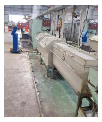
This bath is used for the copper coating process of the wire which comes out from the wet drawing line. Cooper coating bath consists of 3 units. Each unit has a circulation pump. Wire is cleaned by air valves before leaving each bath.
