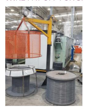
Wire pay off machine is mounted on a vertical column as seen on the picture. There are guiding pulleys that takes the wire from the spool located on the flange.
