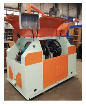
This machine is used for the cleaning of the wire that comes from the descaling machine as the surface of the wire has been cleaned away from the particulars roughly, to make fine surface mechanical cleaning to clean the hot, stuck particulars, this brushing machine is used.
