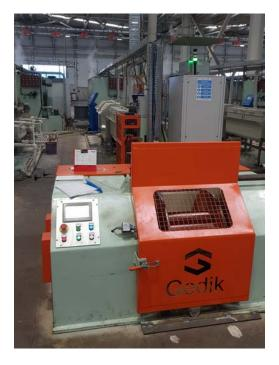
The wire on the drawing machine is electronically and mechanically synchronized and wound on the spool which is located on wire winding machine.
