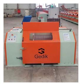
The wire on the drawing machine is electronically and mechanically synchronized and wound on the spool which is located on wire winding machine.
