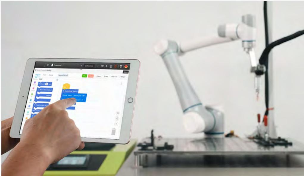
Through the leading full trajectory, the user can drag the robotic arm, quickly generate some positions or trajectories, and then generate various required welding procedures through simple graphical programming.
